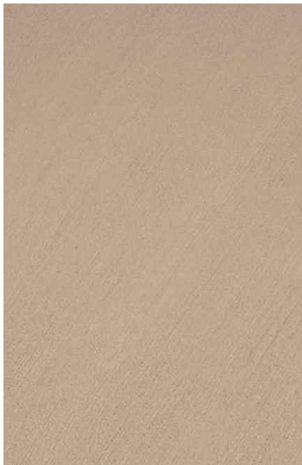
Material: Insitu Concrete Colour: Creme Base Location: Circulation Pathway
